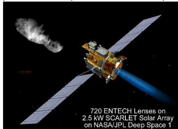
Fig. 2. SCARLET Array on NASA/JPL Deep Space 1 Probe (1998-2001).
