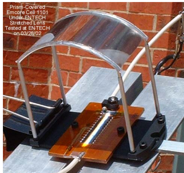
Fig. 5 – SLA Module for Lear/LAPSS Testing
