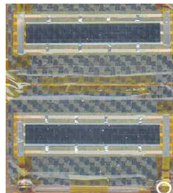
Figure 9 - Stretched lens array module after testing
