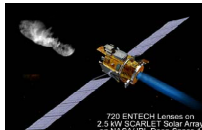
Figure 5. SCARLET Concentrator Array on Deep Space 1
