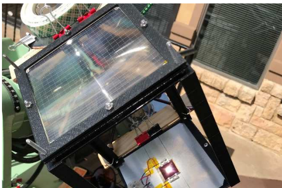
Fig. 12. Silicone Lens with Embedded Titanium Mesh
