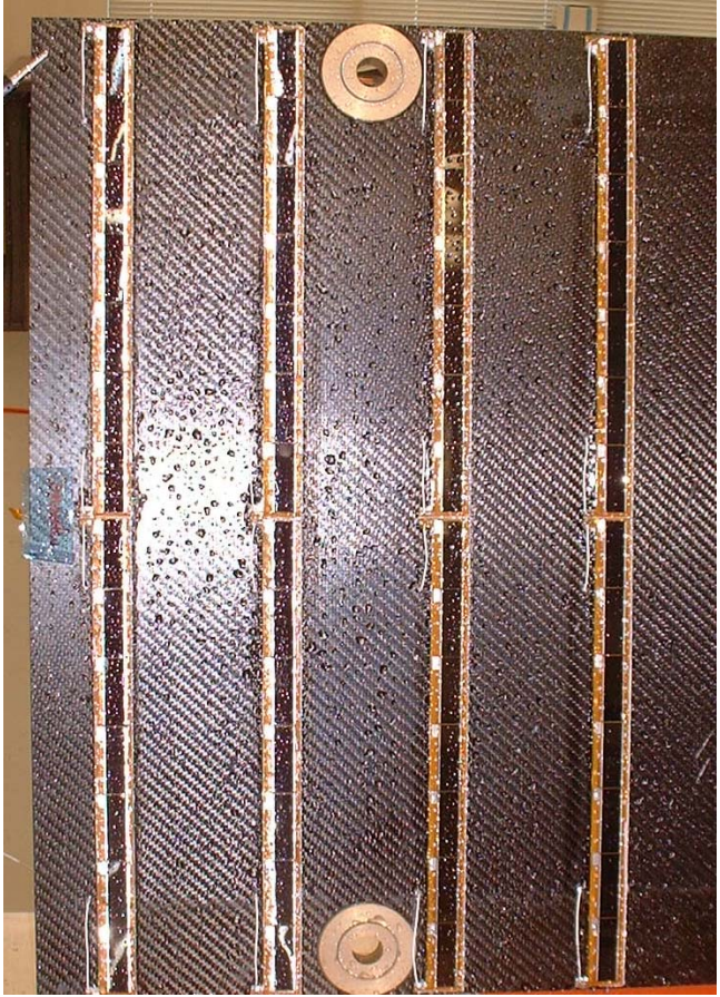
Figure 8 – Photovoltaic Receivers Undergoing 500 V Wet Hi-Pot Testing
