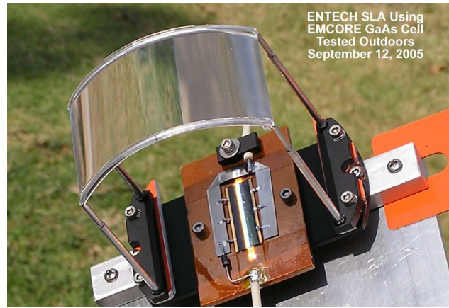
Fig. 4. Stretched Lens Array (SLA) Prototype Using a Single-Junction GaAs Cell Under Outdoor Sunlight Testing.
